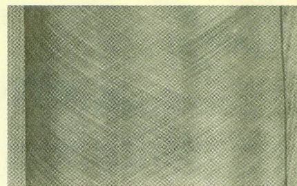
Fig. 2-33—A cross-hatch pattern as shown should be obtained by moving hone up and down cylinder bore as it is being turned by slow speed electric drill.
